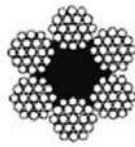
Normal steel wire ropes 6x19+FC According to EN 12385-4
