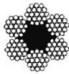
Normal steel wire ropes 6x19+FC According to EN 12385-4
