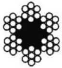
Normal steel wire ropes 6x7+FC According to EN 12385-4
